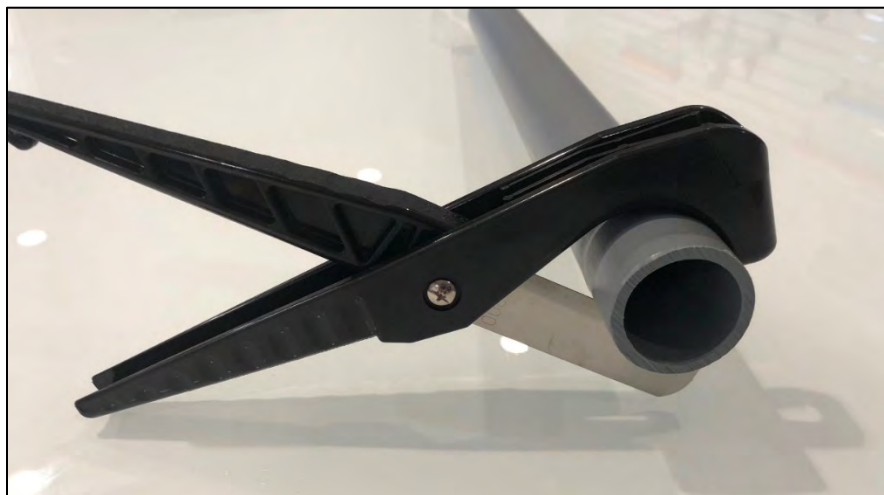
Figure 17b: Tubing cutter for smaller diameter conduit, in use
