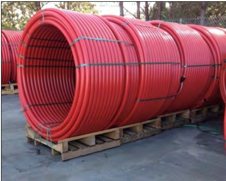
Figure 11. Palletized coils stored horizontally on level ground.
