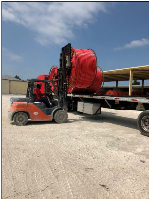
Figure 6. Lifting a reel by the spokes through the center of its drum/hub.
