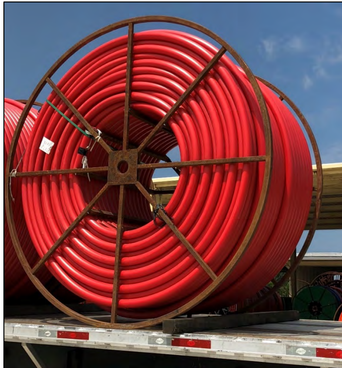
Figure 3. PE conduit on a typical steel reel with temporary blocking to prevent movement during loading/unloading
