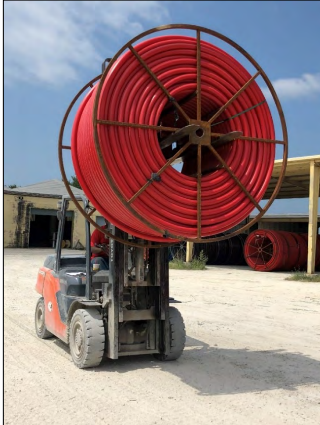
Figure 7. Lifting a reel by the spokes through the center of its drum/hub.
