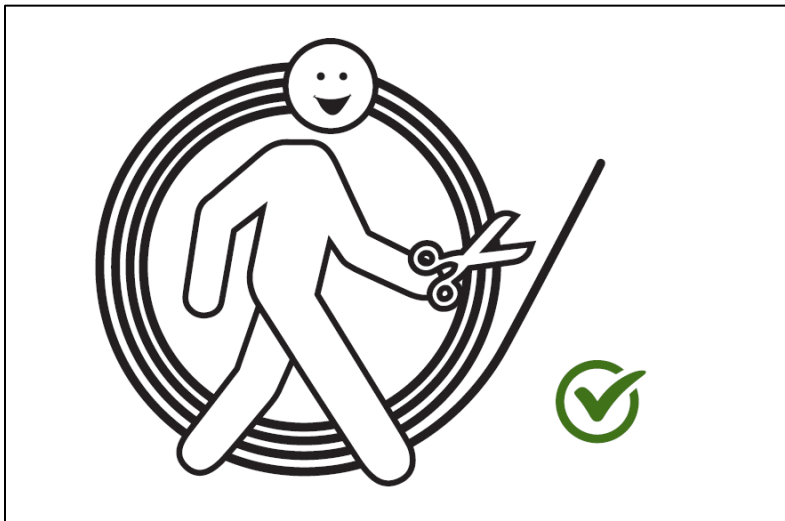
Figure 14. Standing to the side of the reel or coil of PE conduit while cutting it open to prevent injury
