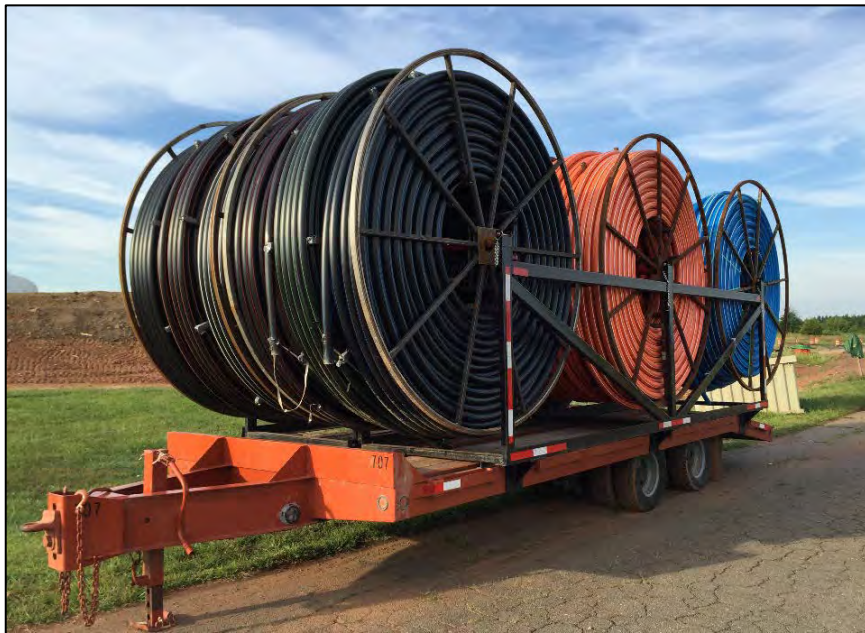
Figure 1. Typical HDPE Conduit on reels, loaded on a trailer
