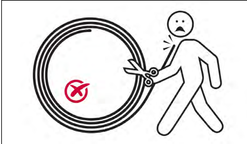
Figure 13. Incorrectly standing in front of the coil of PE conduit while cutting, exposed to injury for rapid unwinding (spring-back) of the coil. Worker is exposed to potential for injury due to sudden spring-back of a reel of PE conduit.
