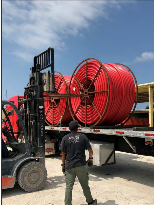
Figure 5. Lifting a reel by the spokes through the center of its drum/hub.
